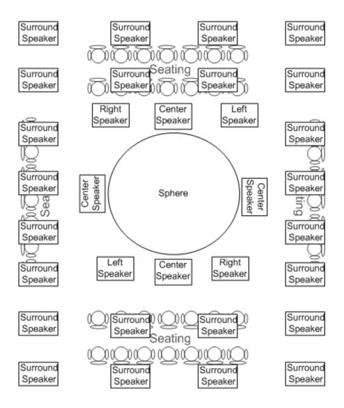
In illustration #6, loudspeakers that are marked "surround speaker" are used for the surround channel and microphone amplification.
