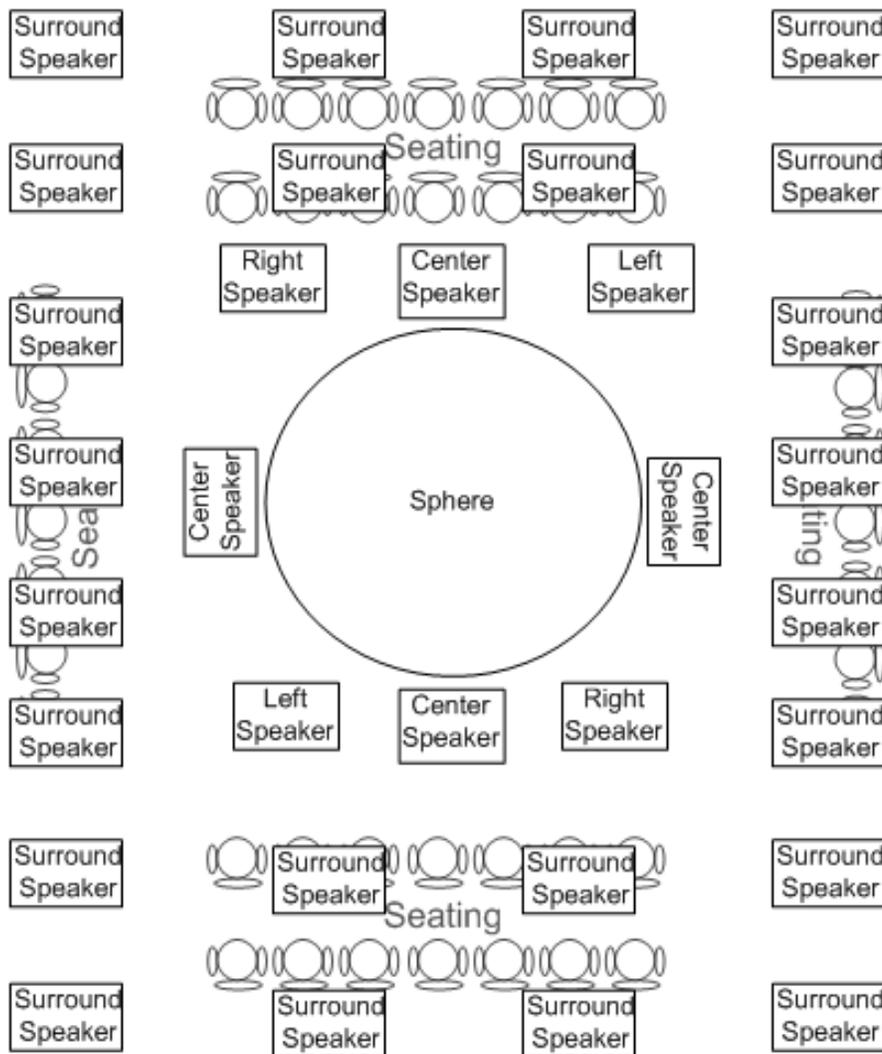
In illustration #6, loudspeakers that are marked “surround speaker” are used for the surround channel and microphone amplification.
