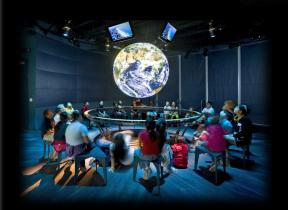
NOAA's Science On a Sphere® uses high-speed computers, projectors, and advanced imaging techniques to create the illusion of a planet, the Sun, a moon, or any other celestial body rotating in space. Weather and other geophysical data can also be shown moving across the surface of the Earth and other planets.
